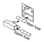
Slo Blo fuse T1.25A is in the case, integrated with power supply socket. There is one spare fuse inside.
